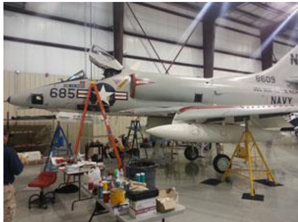
The Foundation A-4 Skyhawk during a phased inspection.
